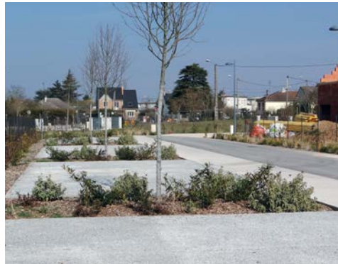
Parking lot in pervious concrete pavement, Dreux (France) © CIMbéton
