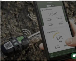
SMARTROCK<sup>III</sup>, EDUCATION, FEATURED ARTICLE Monitoring Concrete Temperature with Wireless Sensors
