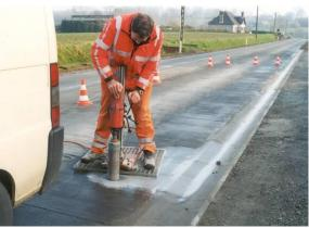
E.g.: ...heavy traffic allowed when the average compressive strength on 3 cores reaches 40 MPa...
